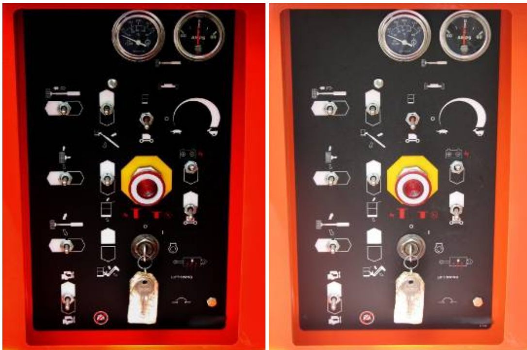
Figure 2.3a: Examples of base controls
